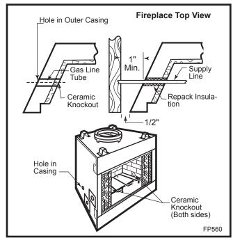
Fig. 26 Gas line access.
